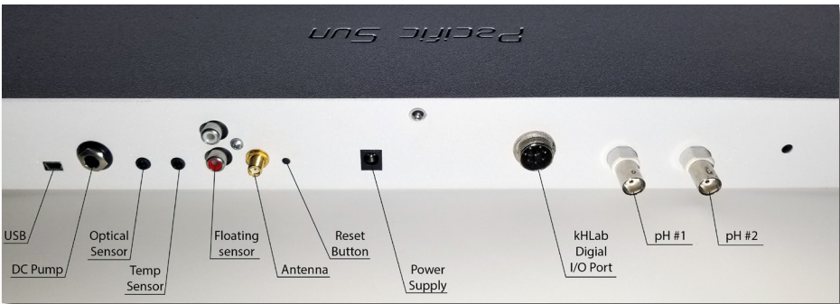
Kore 7th Dosing Station back panel
