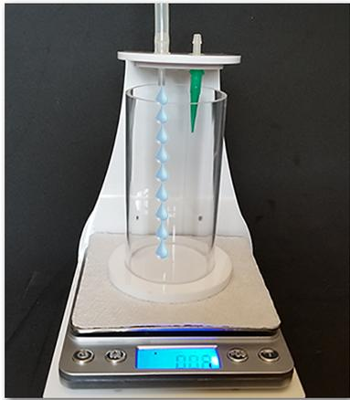
**4** Make sure the supplement is dripping to the measuring cylinder.
